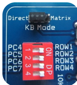
Figure 34. Setting LCD DIP switch (character LCD) in 4 Bit mode
