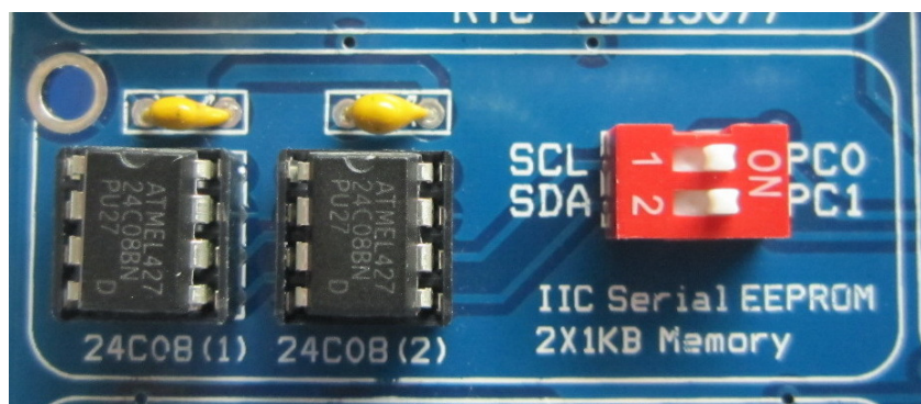
Figure 23. Serial EEPROM unit real PCB view.
